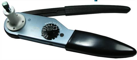
This solid barrel crimping tool has eight indent hand crimps for 12-20AWG Solid Contacts. It is compatible for DT, DTM, DTP, DTHD series and other Deutsch industrial connector families. For use with solid contacts only.
